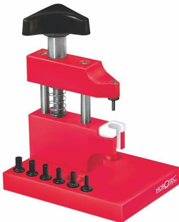
**HOROTEC FOR REMOVE PUSHER W/ 7 PINS**
