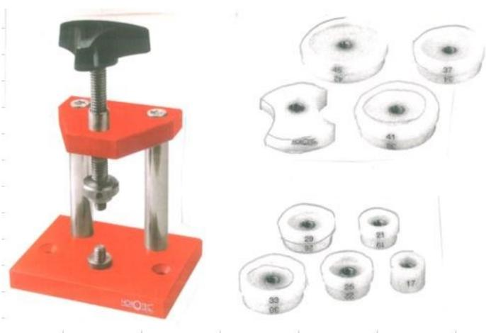
**MICROPRESS FOR SNAP CASE WITH 9 DIES**
