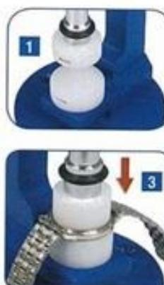
1) MOUNT THE CORRECT DIES ON TOP & BOTTOM
